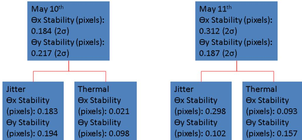
3. The largest boresight instability is from jitter, especially in the  $\Theta_x$  (roll) direction.
