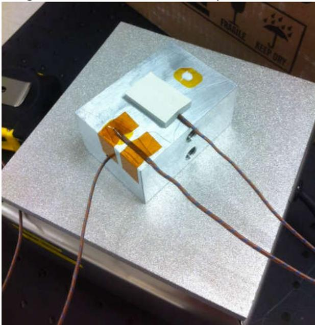
For the comparison, a reference thermocouple was potted into the block using thermally conductive epoxy. The 3 mounting techniques compared were
