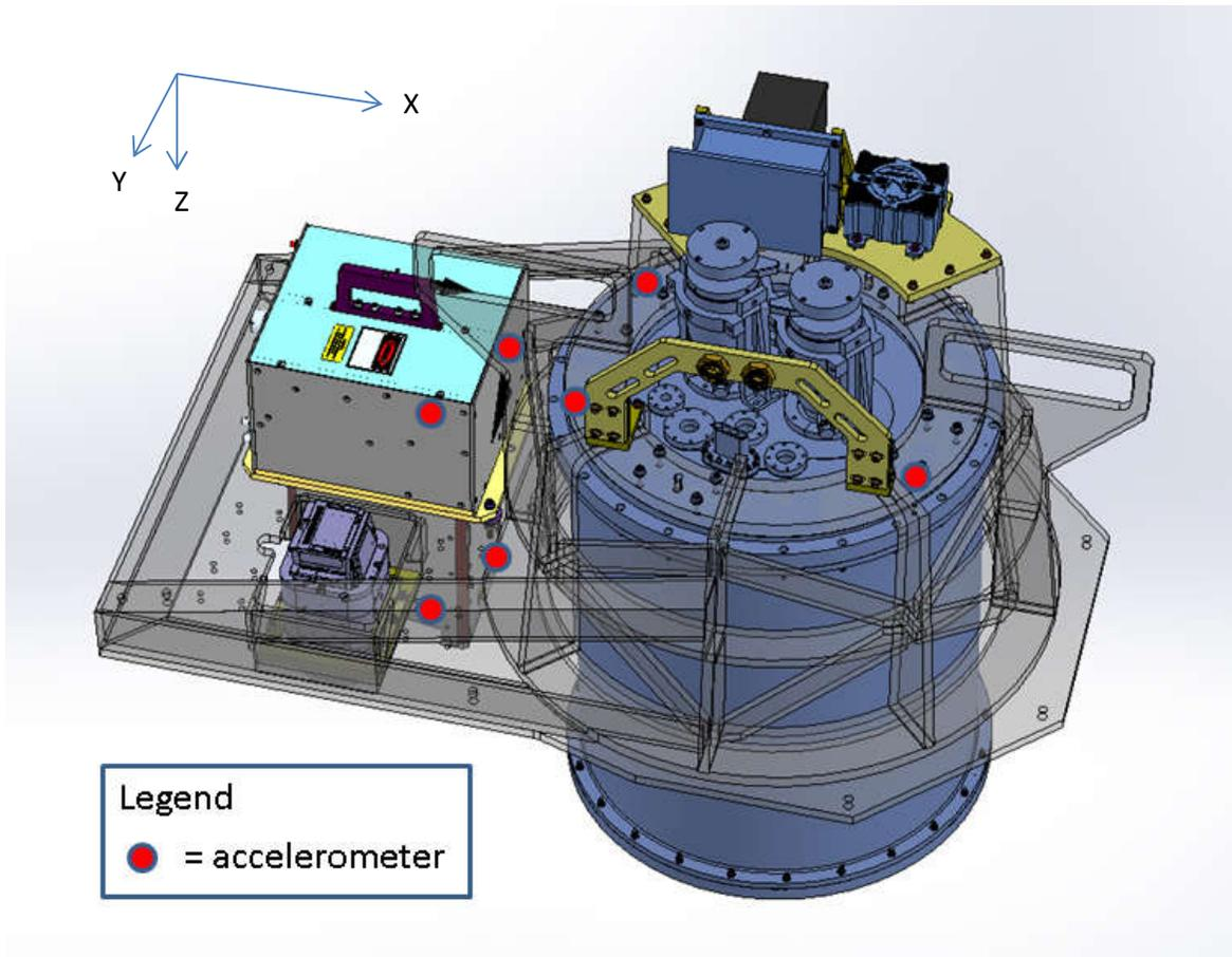
For any rigid object, the periodic angular displacement can be measured by attaching two accelerometers A0 and A1 separated by a distance  $d$ . The periodic angular displacement is
