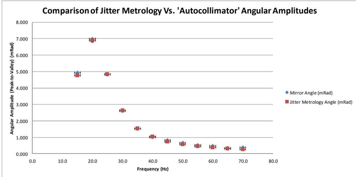
This test served mostly as a check for systematic errors. The first data point was at 15Hz, right at the filter passband, so ignoring that point, the standard deviation of all of the discrepancies in the two measurements is  $46\mu\text{Rad}$ . The actual placement of the accelerometers on the PIM is further apart than on the validation, so the results will be slightly more accurate.
