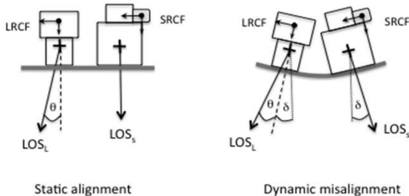
Dynamic misalignments can occur over a variety of amplitudes and frequencies. Here is a list of the relevant frequencies
